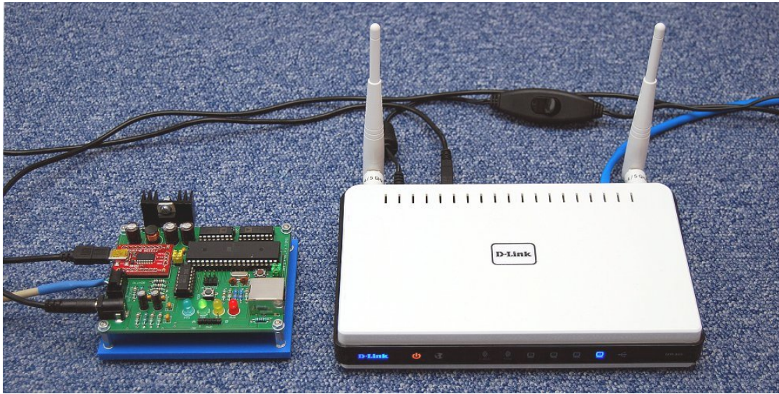
Figure 68: Controller board PCB 6 Version 7 connected to a D-Link DSR-825 router running OpenWrt as a client bridge
