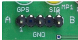
Figure 4: The Measuring Point MP1 of the controller boards Version 6 and Version 8usb
