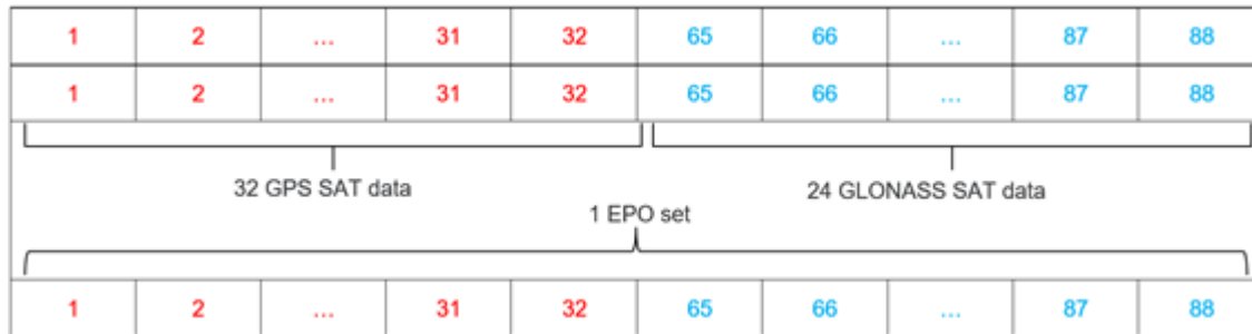
Figure 2. GPS+GLONASS EPO Data Format
